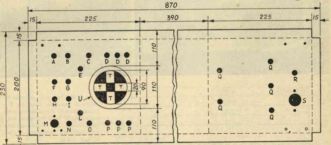
A = SINCRONISMO; B = CENTRAGGIO ORIZZONTALE p2; C = AMPIEZZA ASSE X p8; D = BOCCOLE ASSE X; E = INTERRUOTORE GENERALE D4; F = BASE DEI TEMPI COMMUTATORE D3; G = FUOCO p4; H = BASE DEI TEMPI p5; I = LUMINOSITA' p3; L = COMMUTATORE AMPLIFICATORE D1; M = PRESA AMPLIFICAT.; N = CENTRAGGIO VERTICALE p1; O = AMPIEZZA ASSE Y p7; P = BOCCOLE ASSE Y. Q = FORI PASSAGGIO ARIA; R = CAVO DI ALIMENTAZ.; S = CAMBIA TENSIONE.
